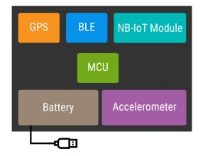
The asset tag comes with dual mode location tracking mechanism - uses GPS based location tracking when the asset or person is outdoors and automatically switches to BLE beacon based location tracking while indoors.
